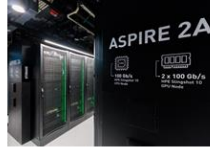
ASPIRE 2A ~10 PFLOPS 100k AMD CPUs 352 Nvidia A100 GPUs
